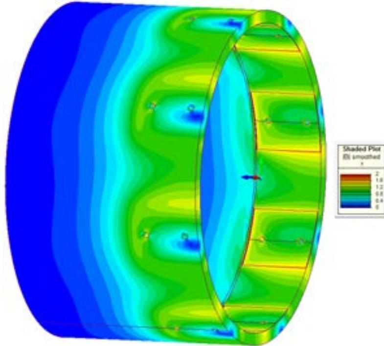
Outer Steel Flux View (Limited to 2 Tesla)
