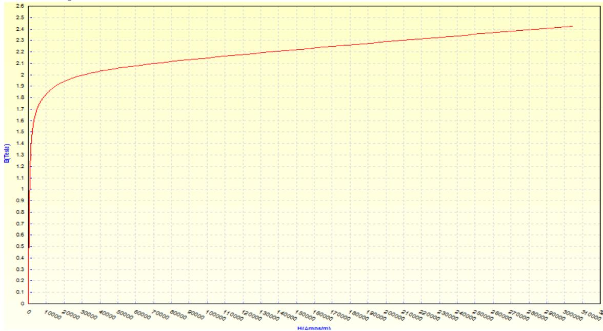
Generic Low-Carbon Steel (1010) – Curve drops off rapidly after 2 Tesla
