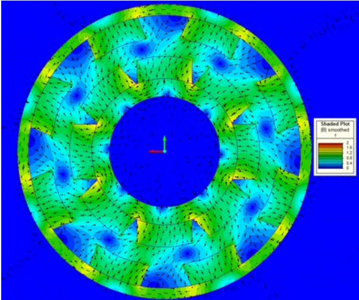
Flux map at drive angle offset of 22.5° at 70°F (limited to 2 Tesla)
