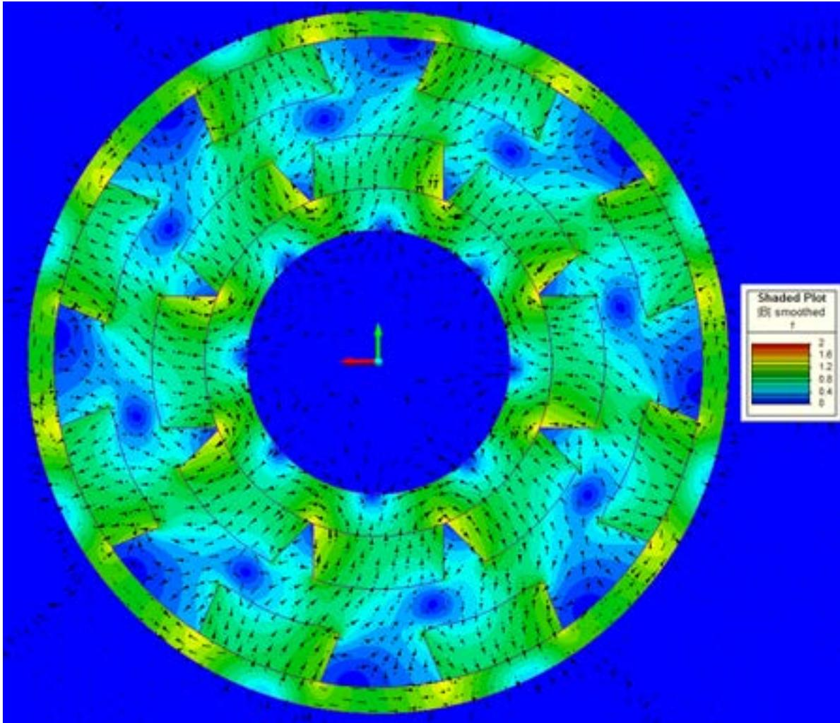
Flux map at drive angle offset of 22.5° at 150°F (limited to 2 Tesla)
