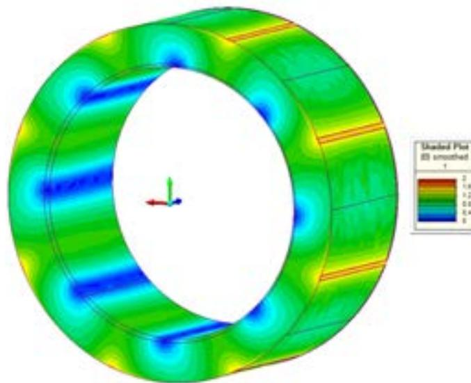
Inner Steel Flux View (Limited to 2 Tesla)
