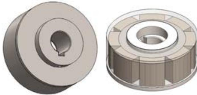
Welded and Completely Sealed Containment Can (with Integrated Shaft Mount)
